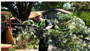
Drag brush to the chipper and stack it so it can be **fed from the side** into the chipper butt-end first. Do not pile too much brush near the chipper. Under no circumstances should any part of the body cross into the infeed hopper.
