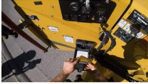
**Before performing any maintenance, make sure the chipper is turned off,** the ignition key is removed and the chip disk or drum is locked in place.
