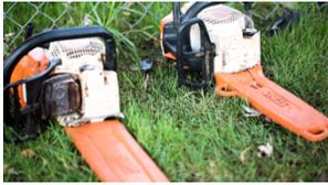
Chain saws are used for limbing and bucking, both common tree trimming practices.
