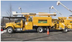
An aerial Lift or bucket truck is the most common equipment used in our operations. Maintaining it properly and inspecting it daily is not only essential but required.
